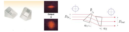
Figure 2.8: (Left) Anamorphic prisms (Thorlabs, PS870). (Right) Geometry of the beam transformation. The entrance side of a prism is often chosen close to the Brewster angle, while the exit side treated carries an anti-reflexion coating.
