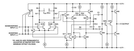
Figure 1. Simplified Schematic
