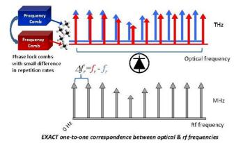
Figure 5.17: Principle of dual comb spectroscopy.
