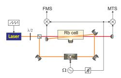
Figure 5.8: Schemes of frequency-modulation and modulation transfer spectroscopy.
