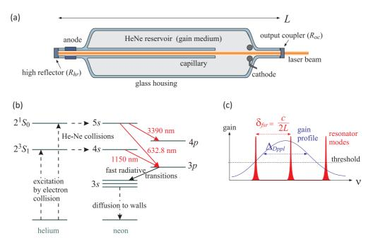
Figure 4.25: (a) Construction scheme of a HeNe laser. (b) Gain and emission profile. (c) Optical pumping scheme.
