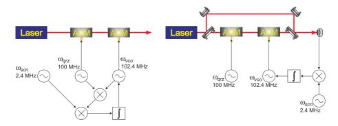
Figure 6.17: Two schemes for laser tuning.
