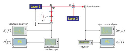
Figure 7.12: (left) Setup for measuring the spectral density of frequency fluctuations  $S_y(f)$ and the Allan variance  $\sigma_y^2(\tau)$  of laser 1 discriminating it at the slope of transmission signal of an optical cavity. (right) The power spectral density  $S_{\mathcal{E}}(\omega)$  can be found as the beat signal between two lasers and either be exhibited on a spectrum analyzer  $S_{\mathcal{E}}(\omega)$  or counted and processed to an Allan variance  $\sigma_y^2(\tau)$ .
