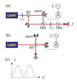
Figure 4.43: Homo- and heterodyning with a Michelson interferometer.
