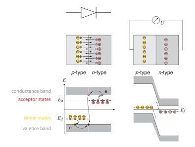
Figure 3.10: Joining a p-type and a n-type doped semiconductor (left) one observes a charge carrier redistribution across the pn transition (right).
