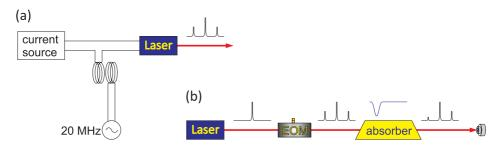
Figure 4.37: (a) Scheme for phase modulation of a diode laser by modulating the drive current. (b) Phase modulation with an external EOM followed by frequency-selective absorption of the lower sideband.
