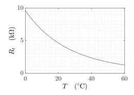
Figure 3.9: Calibration curve for a  $10 \text{ k}\Omega$  thermistor from Thorlabs.
