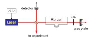
Figure 5.11: Saturation spectroscopy.
