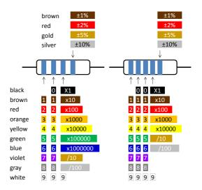
Figure 3.1: Color code for resistors with 4 and 5 rings.
