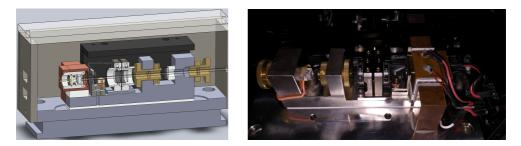
Figure 4.30: (Left) Construction plan of a home-built ECDL lasers in cat-eye configuration. (Right) Side view of the cat-eye laser.
