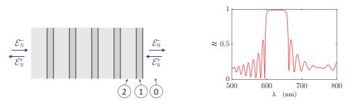
Figure 4.7: (code) Reflection by a high reflecting mirror made of 10 layers with  $n_1 = 2.4$ and  $\Delta z_1 = 80$  nm alternating with 10 layers with  $n_2 = 1.5$  and  $\Delta z_2 = 500$  nm. The absorption coefficient for each layer is supposed to be  $\alpha = 0.2\%$ . The beam impinges from vacuum,  $n_0 = 1$ .
