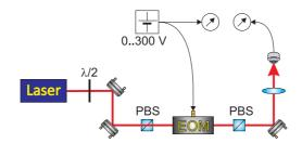
Figure 2.15: Scheme for using an EOM as a Pockels cell.
