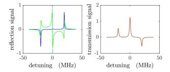
Figure 6.12: (code) (Left) Pound-Drever-Hall reflection signal for  $\theta = 0, \pi/2$ . (Right) Transmission signal.
