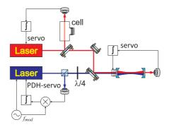
Figure 6.16: Schematic view of a transfer cavity locking system involving three cascaded servo systems for (i) the stabilization of the reference laser to a known frequency; (ii) of the transfer cavity to the reference laser, and (iii) of the spectroscopy laser to the transfer cavity.
