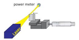
Figure 2.5: Diameter of a Gaussian beam.
