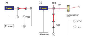
Figure 6.18: Variations on the same theme: (a) Frequency stabilization of a cavity to a laser frequency using the lock-in method. This method is often used for spectral filtering of a laser beam by a transmission etalon. (b) Frequency stabilization of a laser to a cavity using an AOM. The advantage of using an AOM compared to the scheme shown in Fig. 6.10 is, that only the beam injected into the cavity is modulated, but not the beam used for the main experiment.
