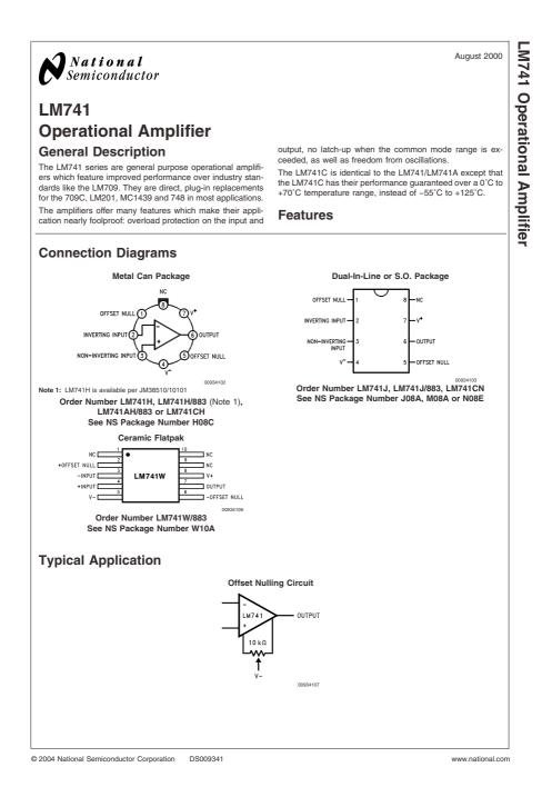
Figure 7.24: Data sheet for the operational amplifier LM741 from National Semiconductor.
