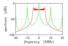
Figure 3.14: (code) Frequency spectra of a phase-modulated carrier frequency for  $\Delta \omega = 5$  MHz modulation excursion and (red)  $\omega = 100$  kHz modulation frequency ( $\beta = \frac{\Delta \omega}{\Omega} = 50$ ) and (green)  $\omega = 10$  MHz modulation frequency ( $\beta = 0.5$ ). Furthermore, a  $\gamma = 100$  kHz resolution linewidth is assumed.
