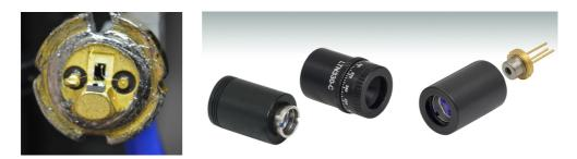
Figure 4.26: (Left) Laser diode with protective housing removed, e.g. using a can opener. (Right) Laser diode collimator.
