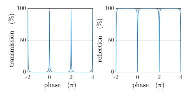
Figure 4.6: (code) Transmission and reflection through a resonator.
