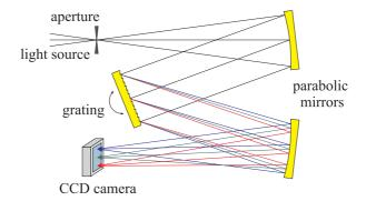
Figure 5.3: Principle of operation of a Czerny-Turner monochromator.
