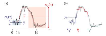
Figure 7.11: (a) Noise can exhibit very different short and long time behavior. (b) Any measurement needs a minimum integration time.
